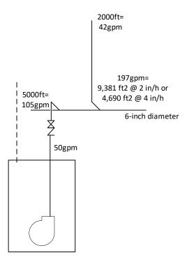
**Conclusion:** Since pipes in Table 1103.2 have been sized according to the flow that they can carry, it is not surprising that regardless of what rainfall is used, the results are the same. Therefore, whether the continuous flow is converted into 24 square feet per gpm and then use the 4-inch rainfall column, or converted into 48 square feet per gpm and use the 2 inch of rainfall column will lead to the same results.
