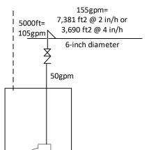
at 2 in/h rainfall, 50gpm are equivalent to 50/0.021=2381 ft<sup>2</sup> (Table D101.1)
